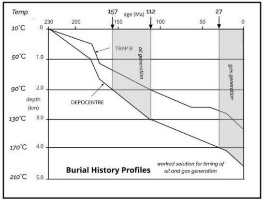
Figure 3. Worked solution for the timing of oil and gas generation
