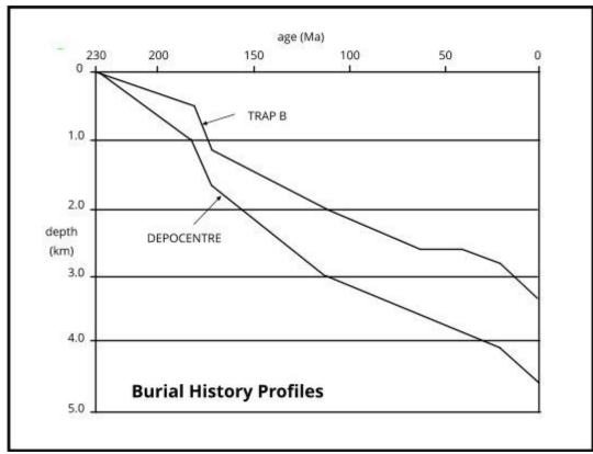
Figure 2 Burial history profiles for the base of the source rock, reconstructed for (a) the depocentre and (b) trap B.
