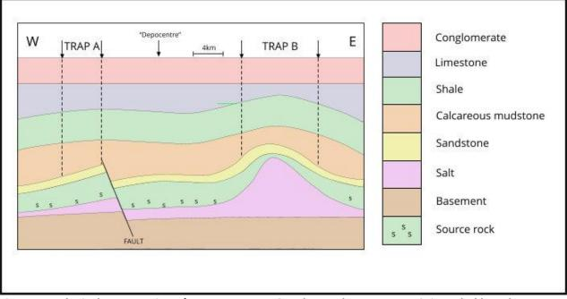
Figure1 Geological cross section. (<u>Note</u>: In traps A & B the sandstone reservoir is sealed by calcareous mudstone)
